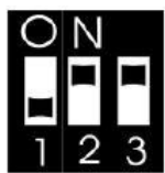
TRANSFER SETTING FOR HOT WATER CIRCULATION
